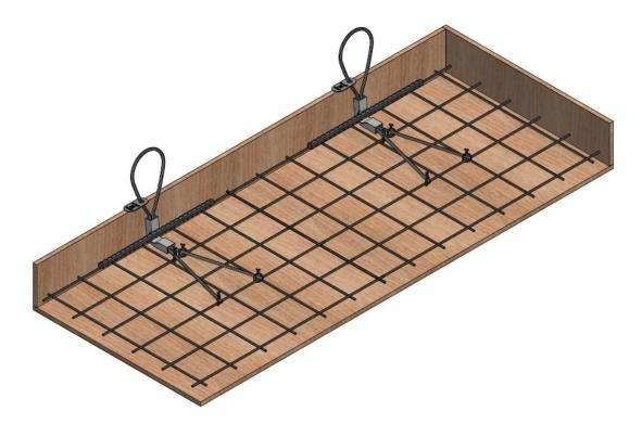
Before concreting the precast element, the bent loops are installed into the mould. To avoid movement during concrete pouring the bent loops must be tied to the mesh reinforcement. An additionally reinforcement bar must be placed above the bent sleeve with pressure contact. Both open ends of the bent loop must be tied at a distance of approximately 300 mm.
